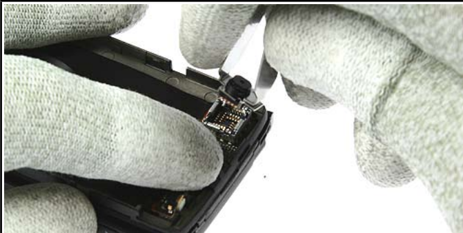
19.) (VGA Camera only RM-78): Release the VGA Camera with the SS-51. Hold the Main Flex near the Camera Socket while removing the camera.
