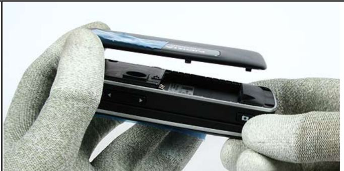
2.) Ensure that no battery is inserted.
