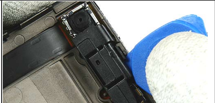
18.) Release the Camera Guide Assy with the SRT-6.
