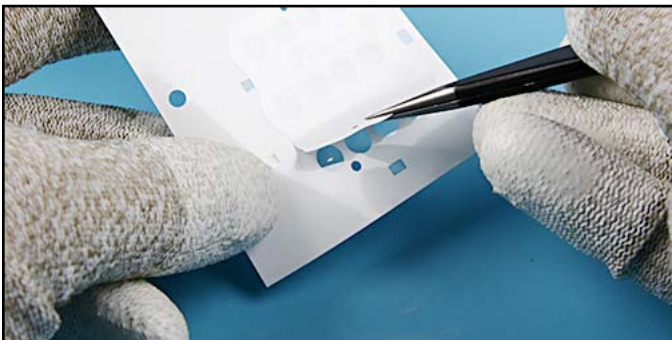
3. Take the new MAIN DOMESHEET from the carrier film.
