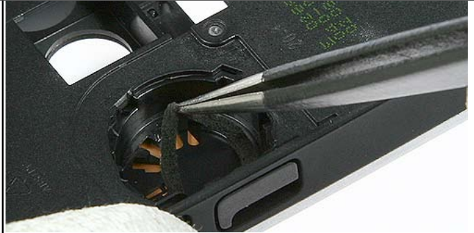
18.) Always remove the residues of the IHF Gasket. Use a new one when reassemble.
