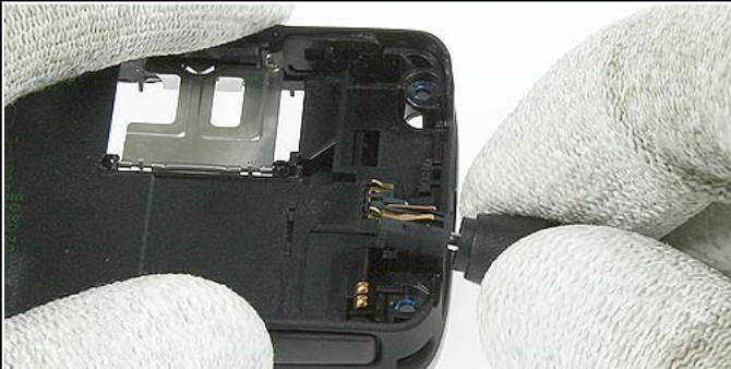
13.) Remove the DC Jack with the DC Plug.
