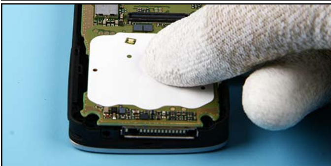
7. Finally, fix the MAIN DOMESHEET all-over.
