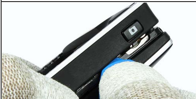
5.) Release the clips of the D-Cover.
