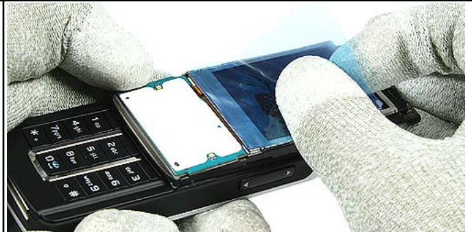
10.) Protect the LCD with a plastic film.
