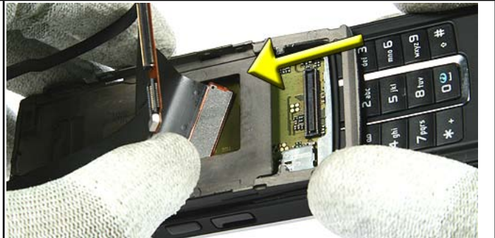
22.) Slot the flex connector through the C-Cover Assy carefully.
