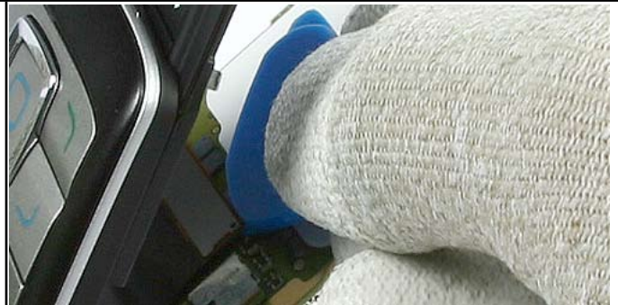
10.) Open the flex connector carefully.
